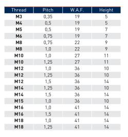
HSS hexagonal die nuts, according to DIN 382, for metric fine threads. Execution:
