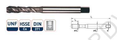
HSS-Co machine taps according to DIN 371, 40° spiral helix, UNF thread, ISO2 (6H), form C lead chamfer, uncoated Execution:
